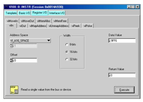
Figure 3-3. Successful viln Access in the VISAIC Register I/O Tab (This Window May Look Slightly Different for LabVIEW Users)
